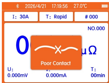
Poor contact Interface
